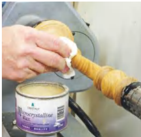
▲ Pic.29 The first candlestick is going to be finished using a traditional beeswax/carnauba mix paste wax. The timber surface is first sealed with an acrylic sanding sealer and then sanded lightly, wax applied and finally buffed to a soft sheen
